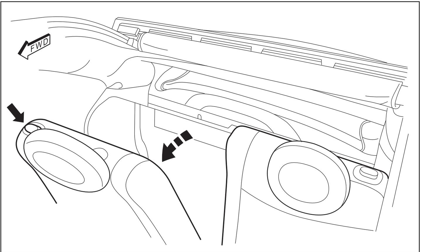
4. Lower the wind screen into position in front of the rear shelf. Carefully insert the left and right mounting brackets into the slot below the rear shelf.
